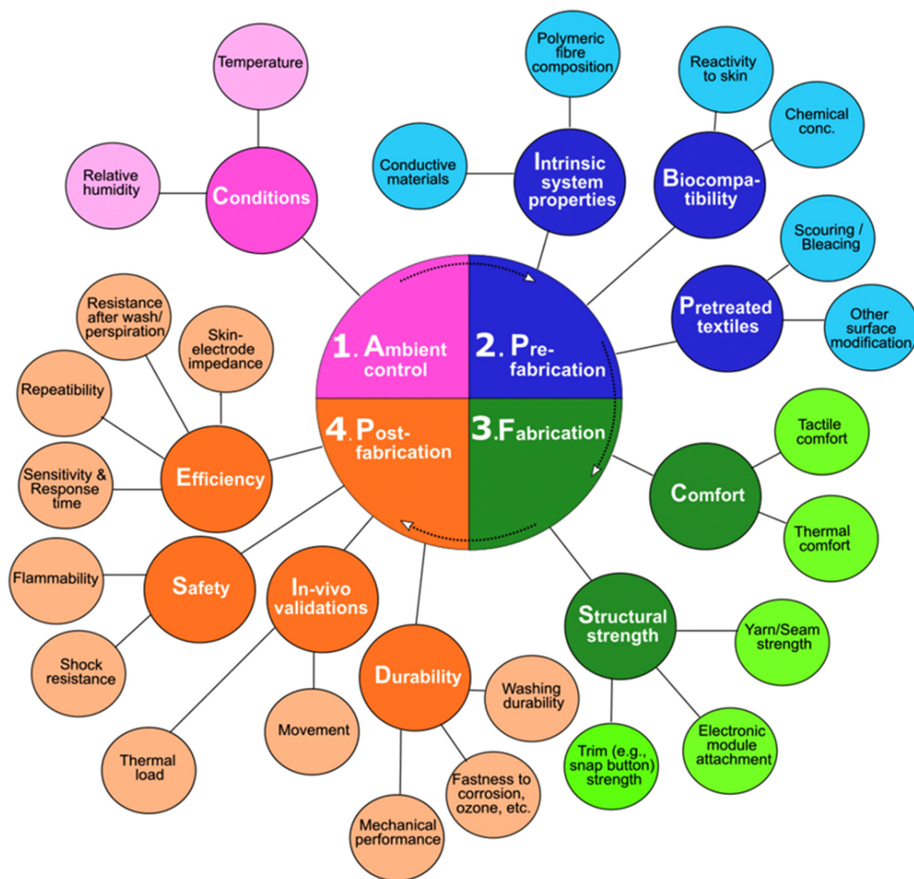
Figure 12. Bubble diagram summarizing the recommended flow for investigating and characterizing textile sensing materials and systems. As textile fiber materials are susceptible to ambient conditions, it is recommended to maintain a standardized ambient condition (1), e.g., relative humidity and temperature, before characterizing the performance of textile sensors. For this purpose, AATCC, International Organization of Standardization (ISO), or ASTM standards for textile materials could be followed. Also, polymer/material composition, biocompatibility (reactivity to skin or concentration of the chemicals), and nature of pretreatments (scoured, bleached, or other surface modifications) conducted on the textile form factors (e.g., fiber, yarn, fabric, or apparel) must be reported before the fabrication of the sensor architecture (2). During the fabrication (3) stages, it is vital to ensure sufficient structural strength of the BSN for robustness and uninterrupted vital signal registration. At this stage, it is recommended to choose the correct fabric structure, yarn tex or setting to maximize the tactile comfort level and minimize the thermophysiological strain on the user of the textronic platform. Scrutinizing the system safety in terms of flammability and electric shock resistivity is highly recommended, while the sensor efficiency and mechanical behaviors are benchmarked during postfabrication (4) in vivo characterization under physiologically relevant thermal loads and movement.
